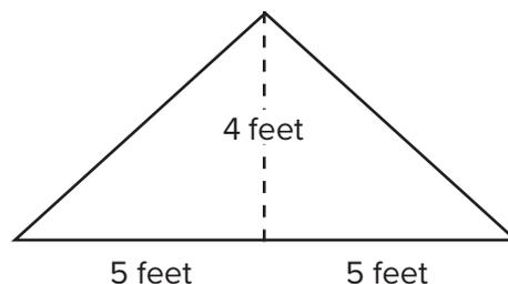
The length of the roof can be calculated by using the Pythagorean Theorem.
